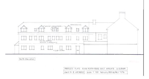
The block has been constructed with the new ridgeline some 0.6m higher than the ridge on the old offshoots, as shown on the north elevation extract from the submitted drawings reproduced below.
