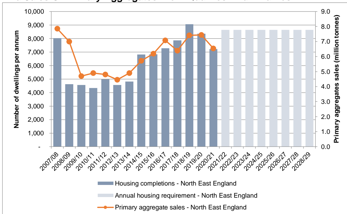
Figure 1 Comparison Between Housing Completions In North-East England And Sales Of Primary Aggregates From Quarries And Wharves
